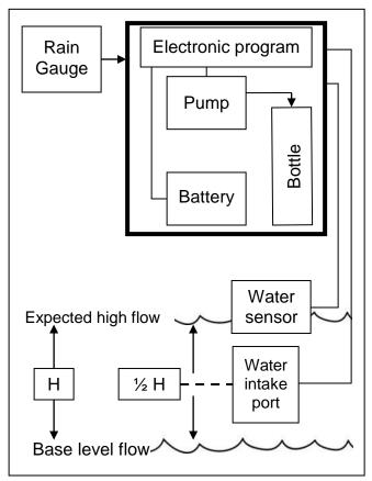
Disadvantage: In setting up the sampler, the installation should keep the difference in elevation from the water intake to the actual pump to a minimum. Peristaltic pumps do not effectively lift water/sediment more than about five feet in elevation above the stream. If your sampler sits on a high bank above a stream, this can be a problem.
